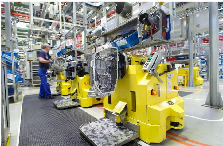
*8-speed automatic transmissions for passenger cars are produced at ZF's location in Saarbrücken.
